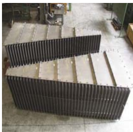
Vane feed inlet distributor
