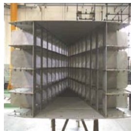
Vane feed inlet distributor
