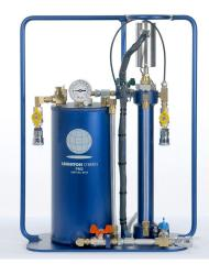
HOW IT Establish safe work area, set up equipment Begin test. Start recording continuous mass readings for wet space that measures any change in mass Inject nitrogen for pressure or draw vacuum into ullage space to measure any change Continue simultaneous testing in pressure of wet and ullage space for relevant period. Technician receives real time results, diagnoses any leaks/issues Data uploaded to cloud and analysed by qualified Digital report sent to customer
